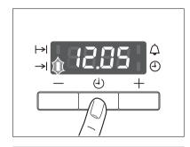
2. Using the + or — button set the desired switch-off time.
